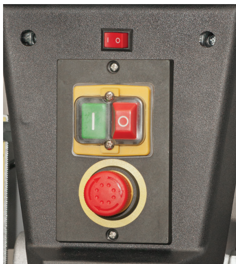
Betjeningspanel for AP32FD MERK: Bryteren for LED-lys sitter over Av/på-bryteren.
