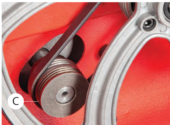
Drivenhet for AW1950B båndsag Totrinns remskive (C)
