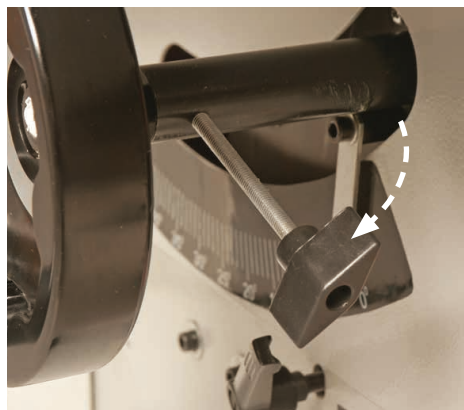
Panel saw rise and fall control butterfly handle lock
