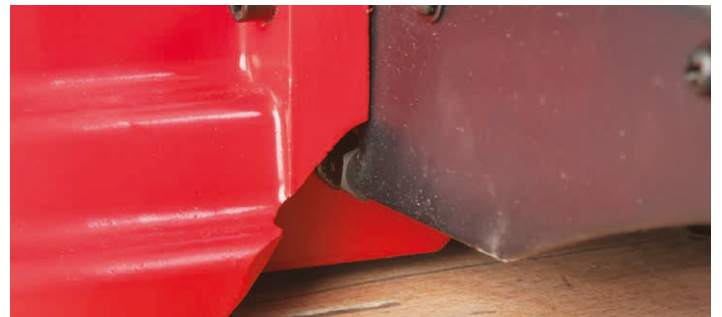
Extension table levelling bolt
