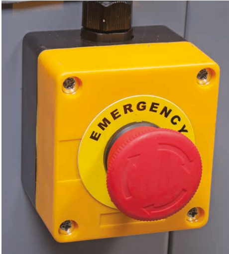
Emergency stop, press to stop the bandsaw
