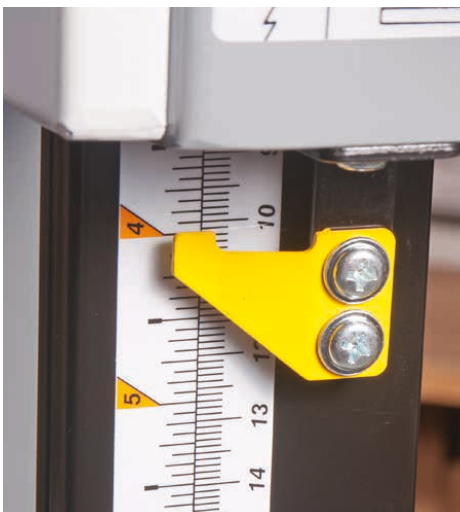
Upper blade guide height scale and pointer
