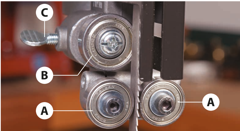
Upper bearing blade guides (A), Rear thrust bearing (B) and rear thrust bearing butterfly clamping screw (C)
