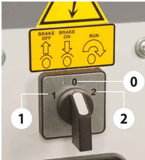
Electro-magnetic motor brake switch Brake OFF (1), Brake ON (0), Run (2)
