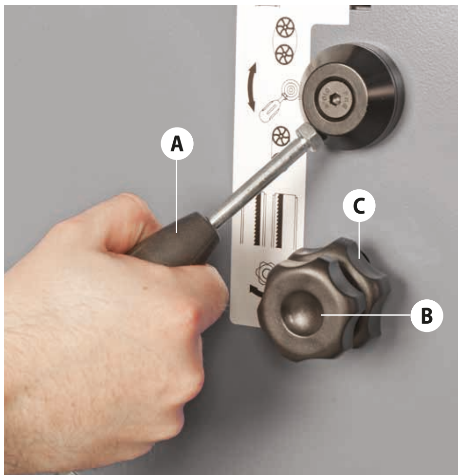
Quick release tensioning blade lever (A), Tracking control knob (B) and locking knob (C)
