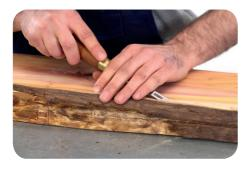
Although you probably love the appearance of the bark on the live edge of your timber, it's advisable to completely remove this bark and sand the edge of the timber back to the good wood. This will allow the resin to bond to the solid material and result in a much more sturdy finished piece.
