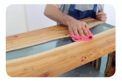
Liberally apply your chosen polishing compound to the satin finished resin and then use a power polisher with a medium to hard polishing pad to polish the surface. Keep topping up the NW1 as needed until it reaches full gloss.
