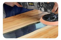
When polishing GlassCast® 50 we suggest starting from at least a 1200 grit abrasive paper finish. We recommend Pai Cristal NW1 polishing compound to polish the GlassCast® 50 because it is a fast-cutting compound designed specifically for hard-wearing plastics like epoxy resin. Additionally, NW1 uses a special low-drag formula which reduces heat build-up whilst polishing. Nonetheless, if you do start to feel heat building up in the resin when polishing you should stop or move on to another area.
