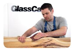
Then use some 80 grit abrasive paper to rub back any loose material left on the de-barked edge to ensure the edge is left as smooth as possible ready for the next stage. Make sure you clean any dust and dirt from the wood using a cloth or vacuum cleaner.
